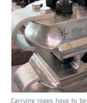
Carrying ropes have to be re-aligned at regular intervals. Our hydraulic power units, winches and rope clamps take care of this hard work with precision - to reliably put ropes with a radius of up to 70 mm and a tensile strain of 160,000 kg in
