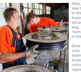
If necessary, the large sheave assemblies, which can weigh up to 2,500 kg, take to the air: Our assemblers dismantle them into several parts directly on the tower. Then they can be easily transported away using a smaller helicopter – this way, the costs are reduced to a minimum. In turn, the assembly takes place in the air via helicopter.
